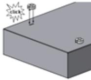
3. Put mains cable through the hole in the luminaire's body.
